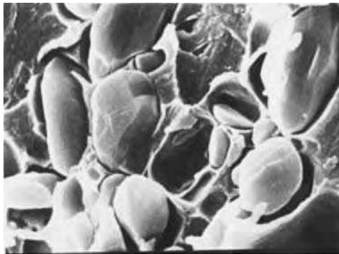
FIGURE 18.4 Polymeric spacer particles in a toughened epoxy resin, revealed by scanning electron microscopy of a cryo-fracture of a sample of the cured resin. (Particle size range 1 to 10 \mu\text{m} .)
