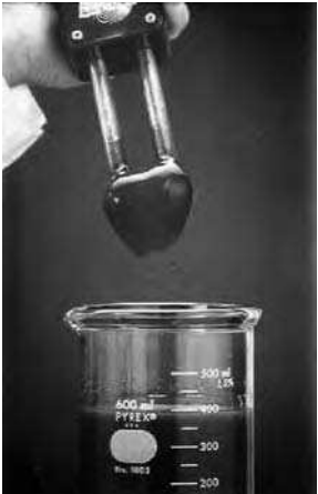
FIGURE 8.3 Magnetorheological fluids—a material with real-time adaptive rheology.
