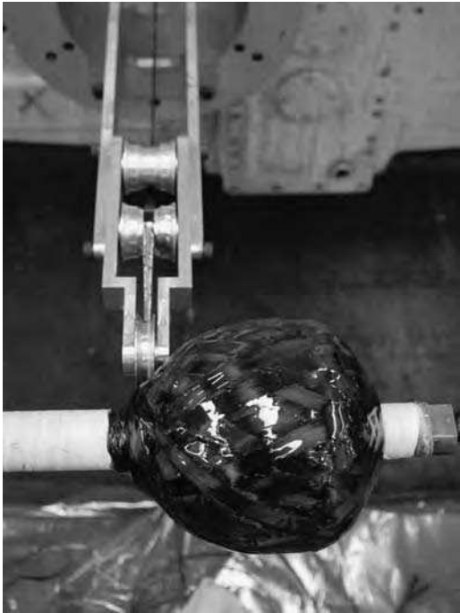
FIGURE 19.4 Filament winding of a CFRP accumulator vessel on a thin-walled aluminum liner/mandrel.
