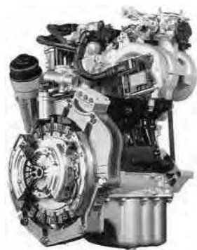
FIGURE 7.7 Multifunctional starter-generator system.
